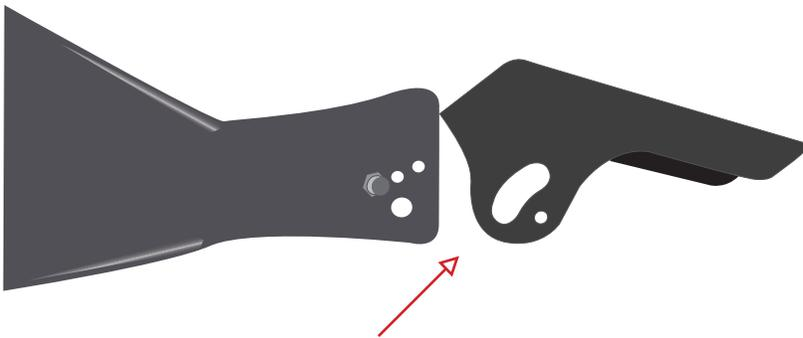
Hook one side of funnel onto the hopper. Second side will be a bit tight, so pull and “snap” into place above the bolt.
