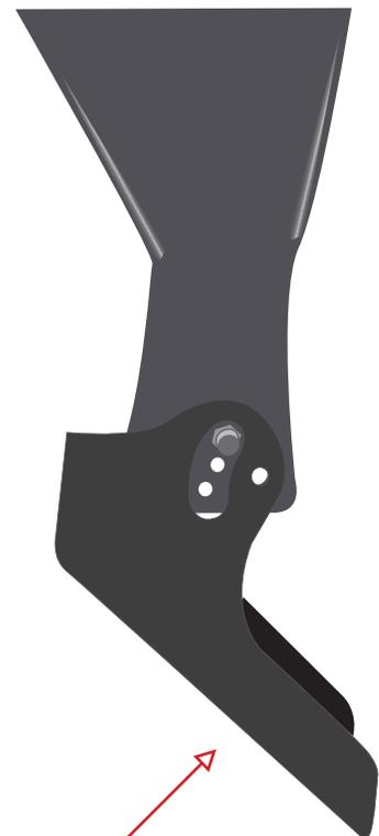
Adjust funnel at a steep enough angle that the activator can move freely up and down, and feed can slide easily down the chute.
